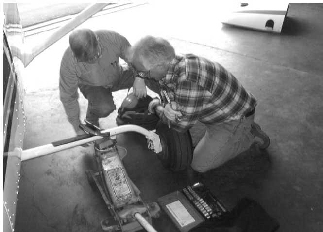
CPA Tech Rep Tom Carr demonstrates correct jacking procedure for an aircraft inspection to Tom Freeman, CPA member.
