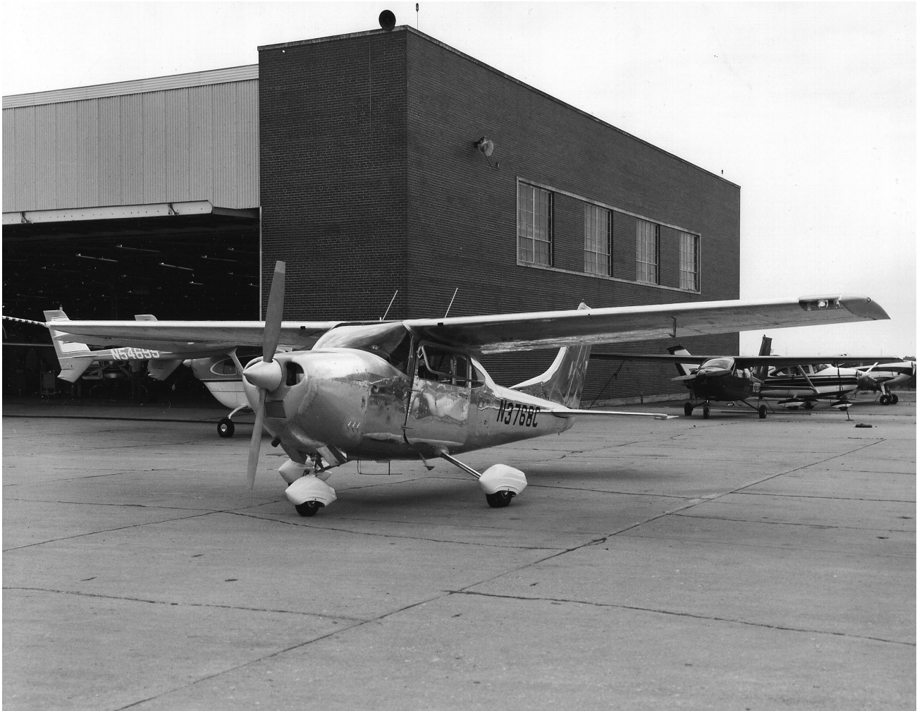
Prototype of a cantilevered wing Cessna 182M. Lack of performance improvement lead the factory to decide not to put a cantilever wing 182 into production.
